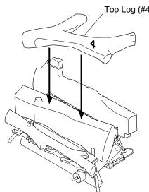
Figure 19 - Installing Top Log
